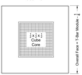
Note: This product complies with NFPA 90A-1B standard 4.3.7.3.2 and 4.3.8.3.2 and is constructed with openings through which a 1/2" sphere can not pass.
