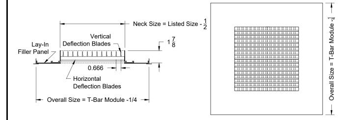
Note: This product complies with NFPA 90A-18 standard 4.3.7.3.2 and 4.3.8.3.2 and is constructed with openings through which a 1/2" sphere can not pass.
